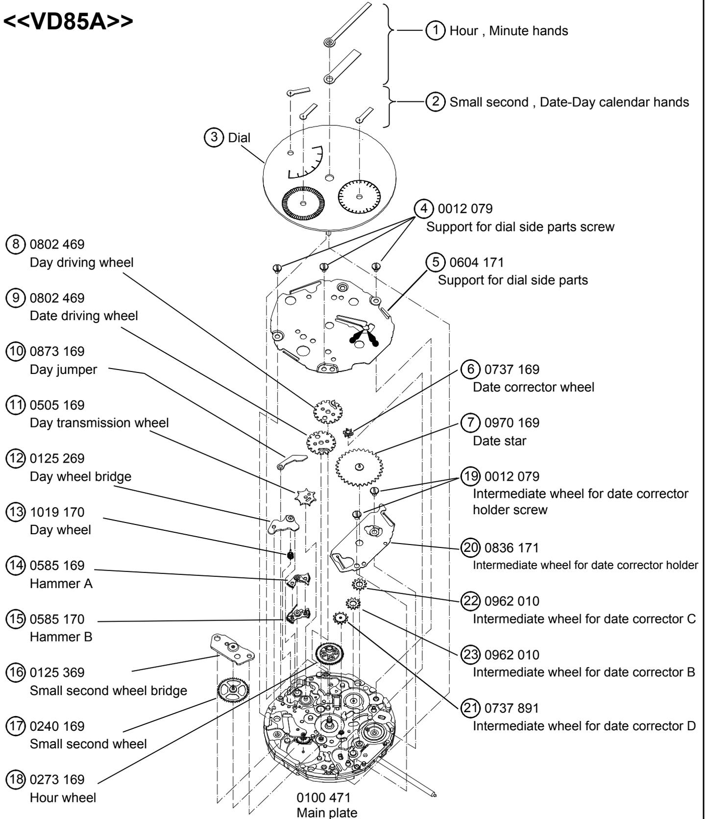
Disassembling procedures Figs. ① ⇒ ②③
