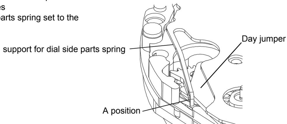
(6) Setting position (Notes at the time of disassembling and a reassembling)
