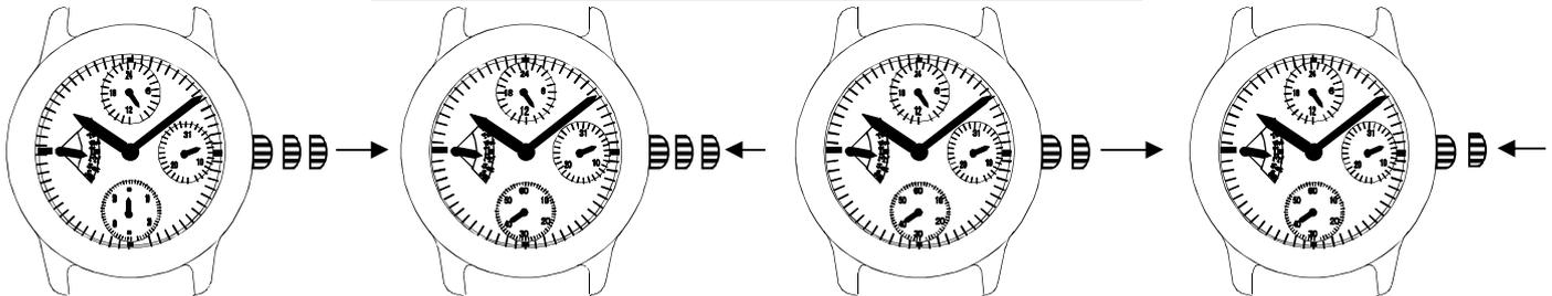
1.Pull out the crown to the second click when the small second hand is at the 12 O'clock position.
