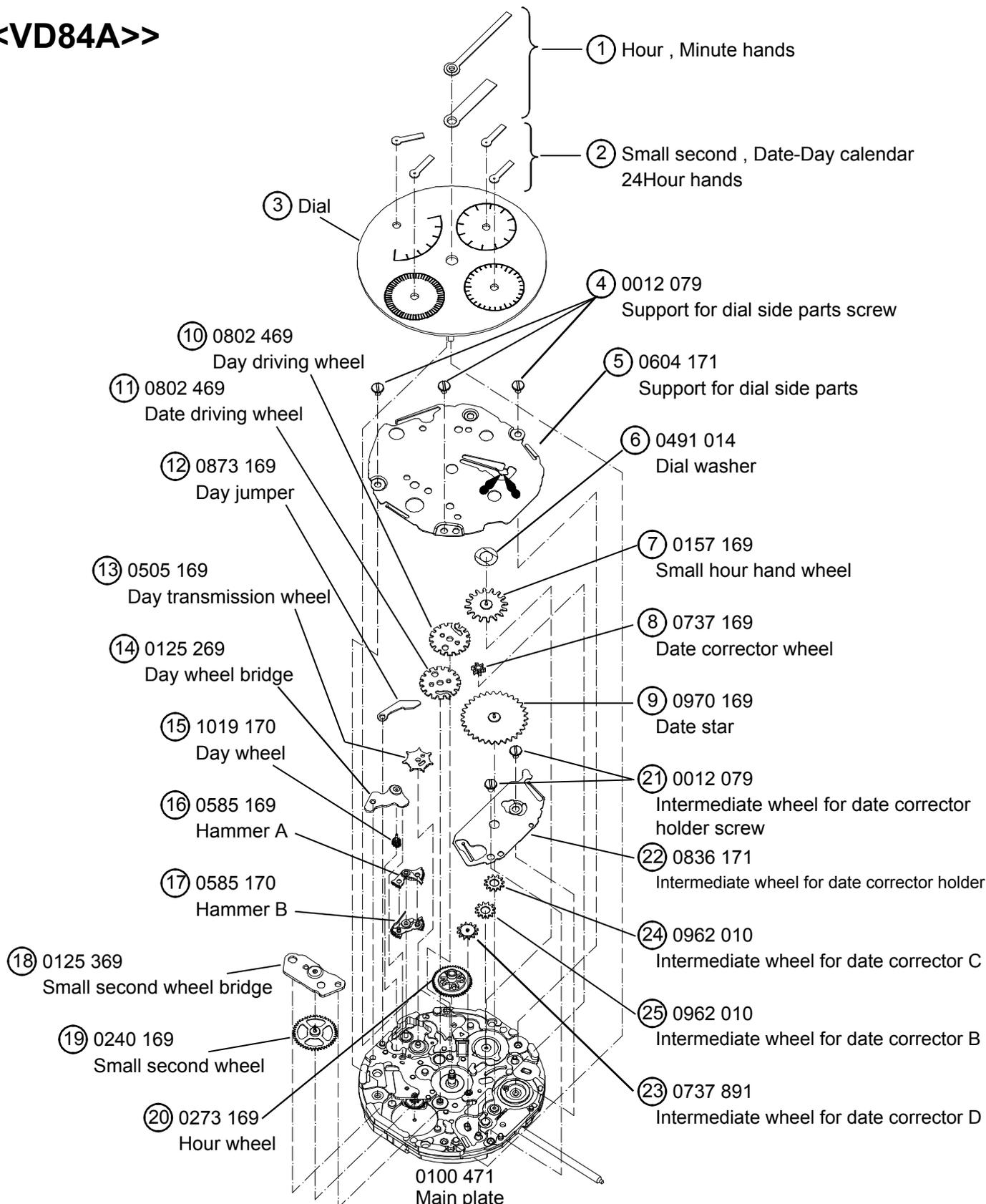
Disassembling procedures Figs. ① ⇒ ②③
